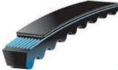
Cogged V-Belt Reduces bending resistance and friction
