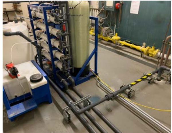
Figure 10: Piping unique to this testbed: metered drain (left), overflow repiped (right)
