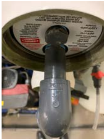
Figure 11: Retrofit to original BDR test unit to add self-cleaning functionality
