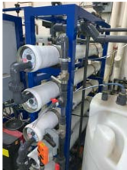
Figure 11: Retrofit to original BDR test unit to add self-cleaning functionality
