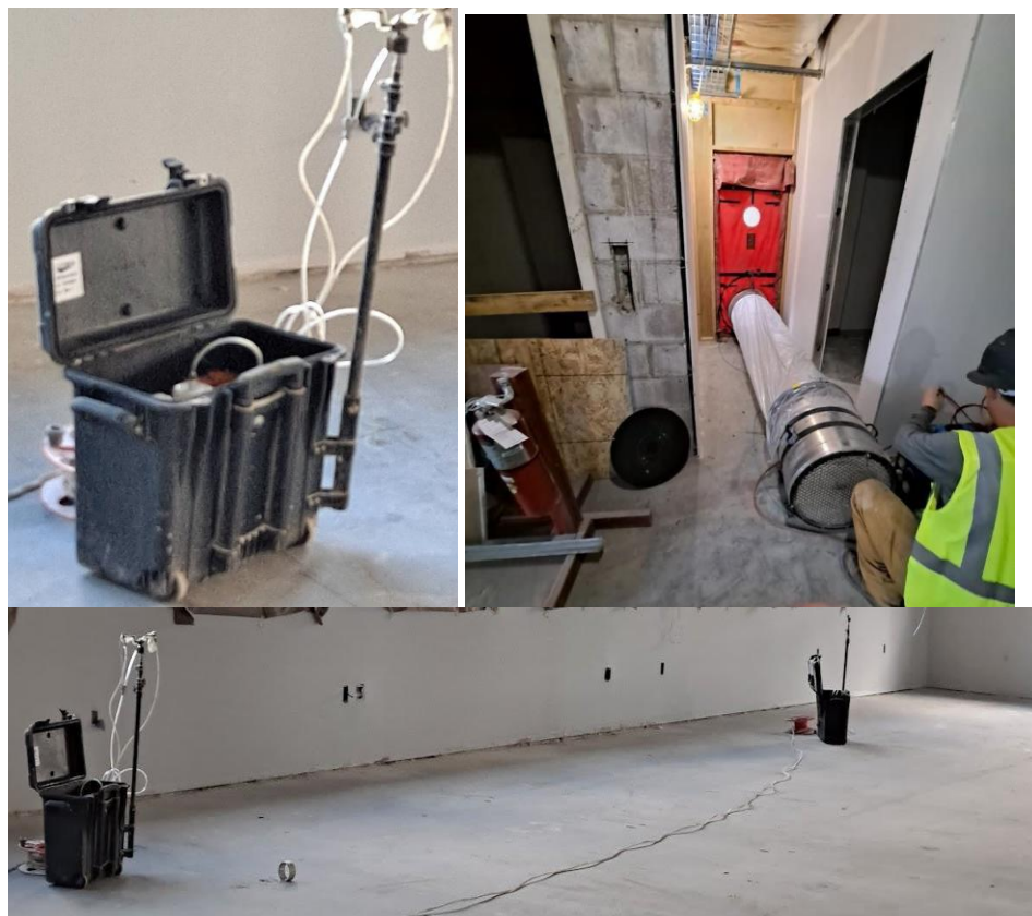
Figure 7. Aerosol sealing station and blower door equipment.
