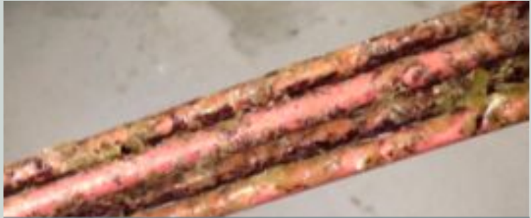
After Non-Chemical Scale Prevention
