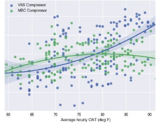
Energy consumed (in kilowatt-hours) per hour when condenser EWT is between 77.5°F and 82.5°F
