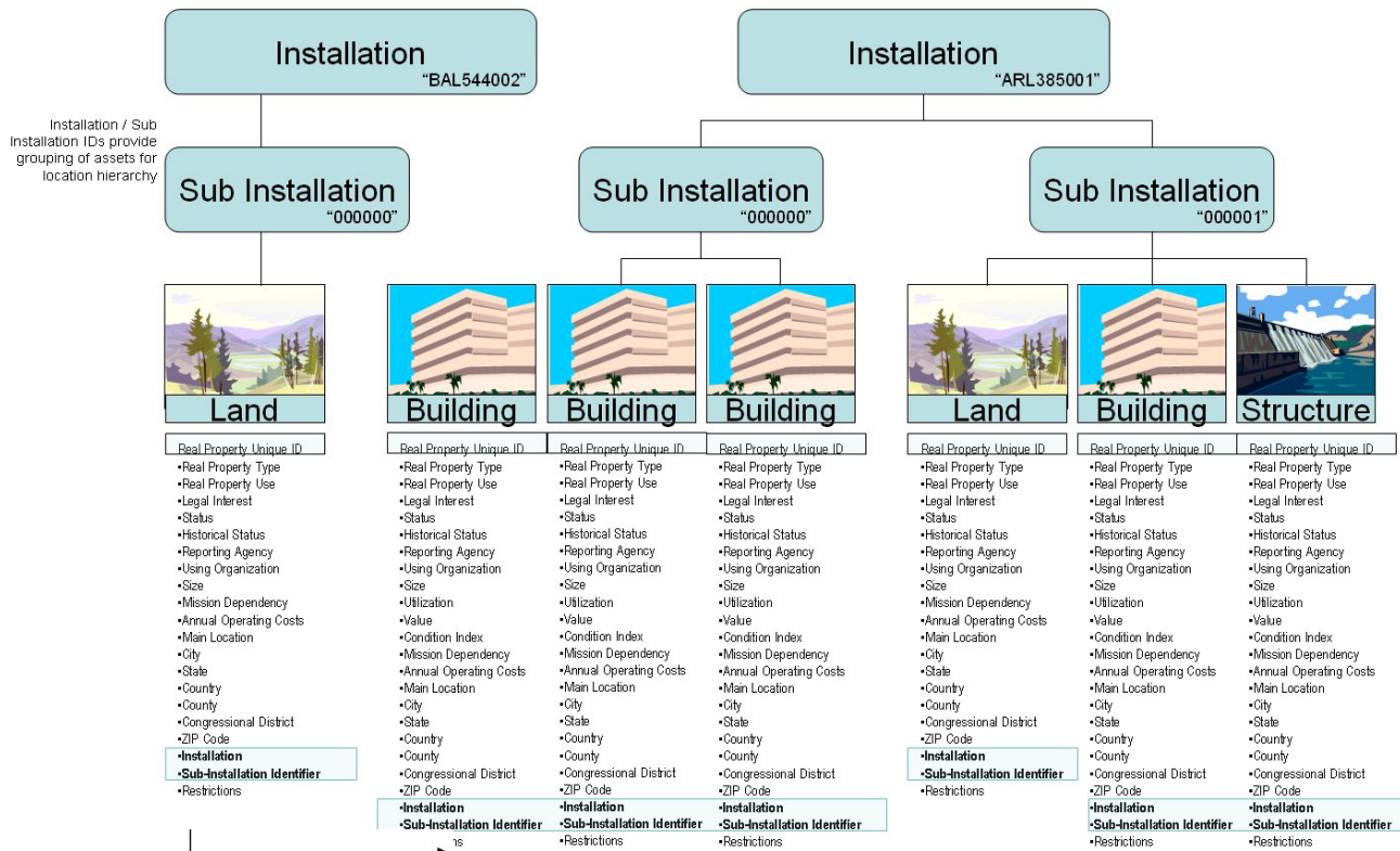
Figure 2: Relationship of Installation/Sub Installation Hierarchy to Real Property Unique ID (each asset record)
