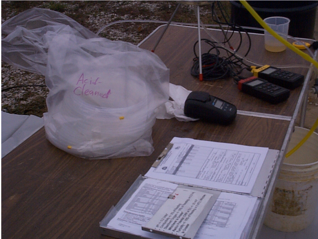
Photo G-9. Acid cleaned tubing per arsenic speciation method requirements.
