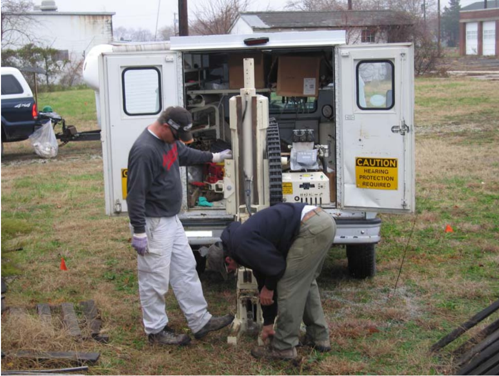
Photo G-5. Direct push soil sampling at 434-SB-05 location.
