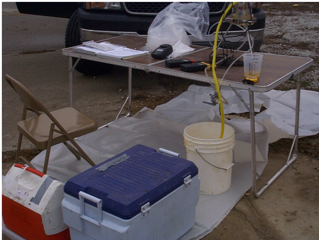
Photo G-10. Low flow sampling rate being determined at 413-MW-03.
