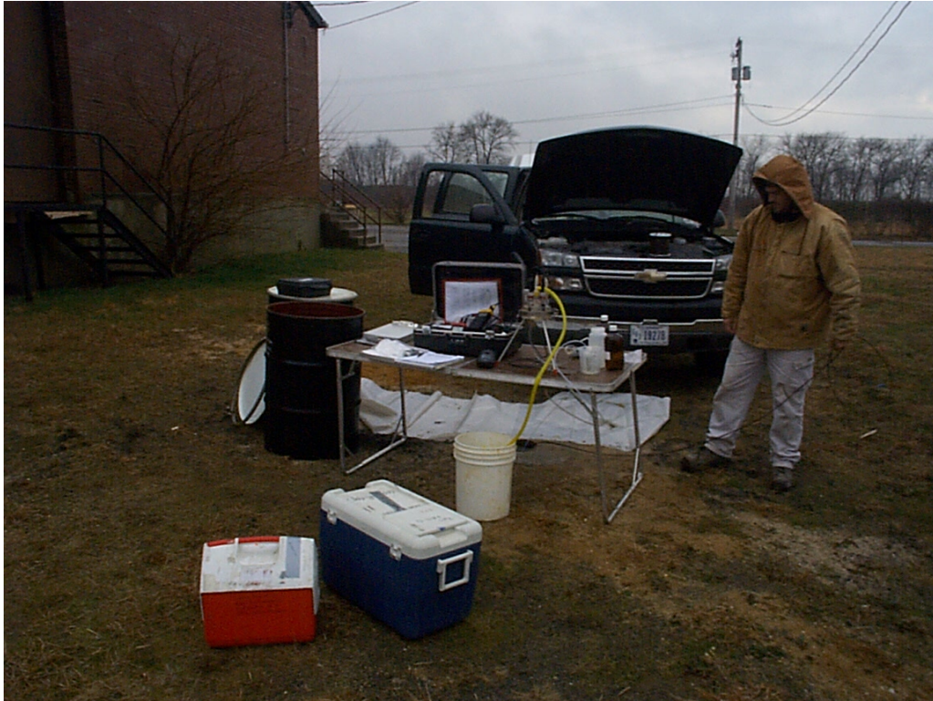
Photo G-14. Purge water collection barrels at 434-MW-02.
