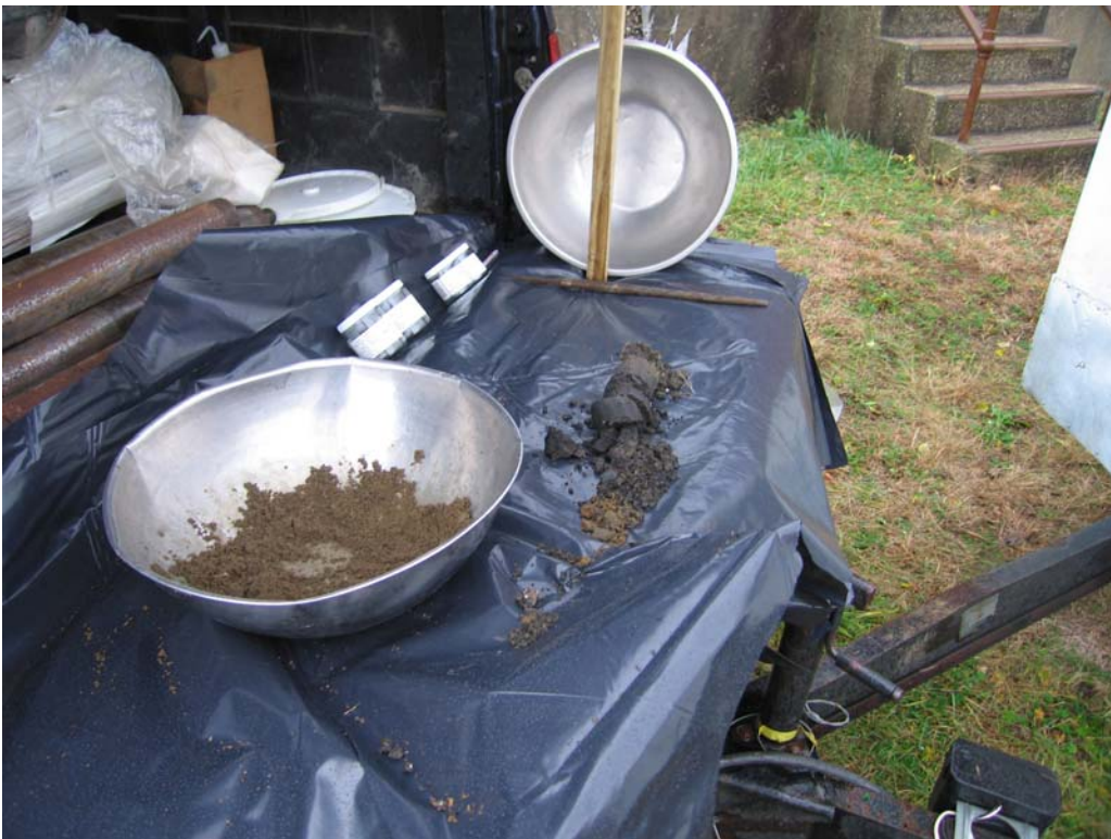
Photo G-2. Composite sample collection and soil logging at 434-MW-01 location.
