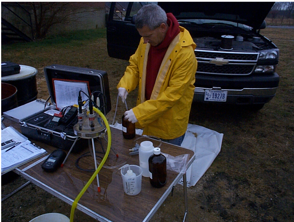
Photo G-15. Excellent turbidity of ground-water sample, the last sample being taken at 434-MW-02.
