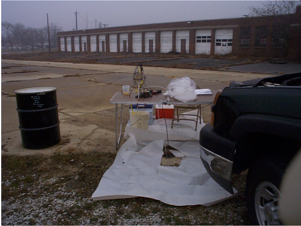
Photo G-12. Low flow ground-water sampling set up at 413-MW-01.
