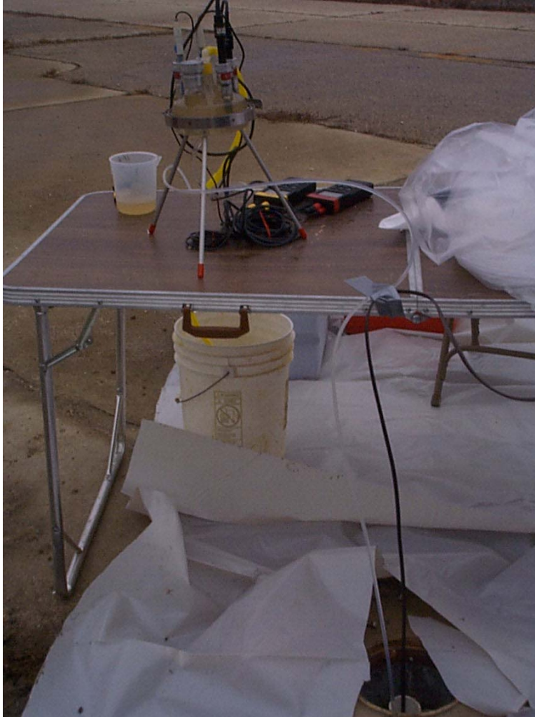
Photo G-11. Low flow chamber utilized for ground-water quality field measurements at 434-MW-03.
