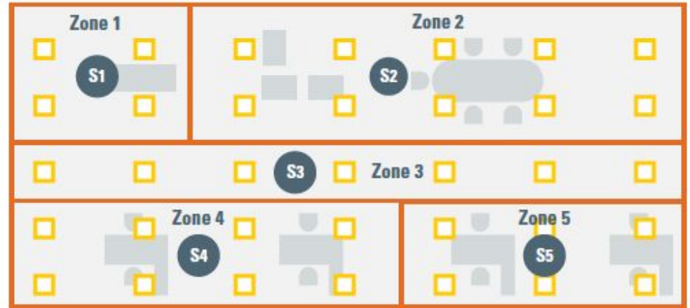
Sensors are Mounted External to Luminaires in Zone-Based Control
