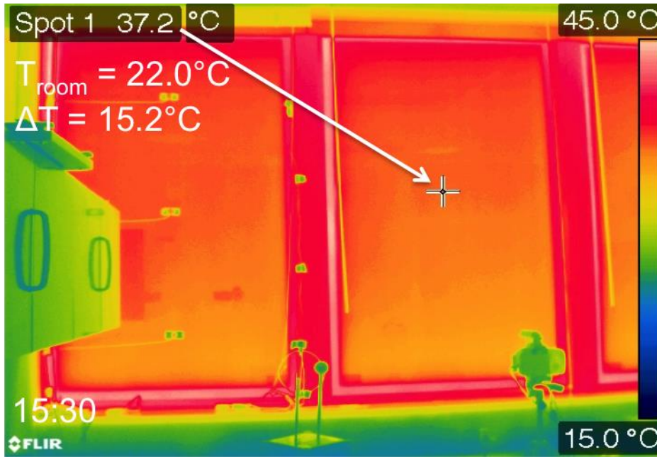
Figure V-28. Infrared false color image taken on April 16, 2016, at 3:30 p.m., when EC window glass temperature was at its peak.
