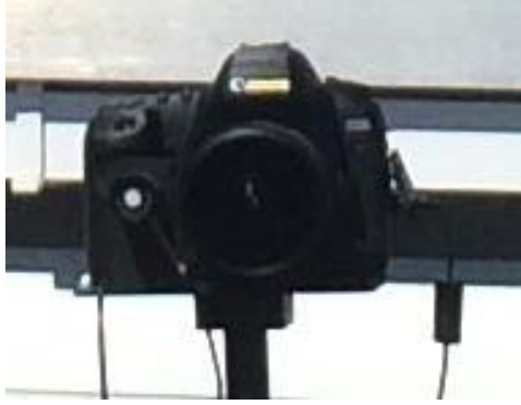
Figure IV-24. Canon 5D Mk II and equidistant 180° angular fish eye lens used for HDR image capturing.
