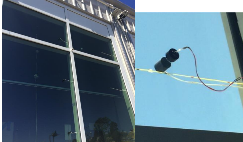
Figure IV-23. (left) Six transmittance sensor positions in a test room. (right) Close-up view of transmittance sensor.
