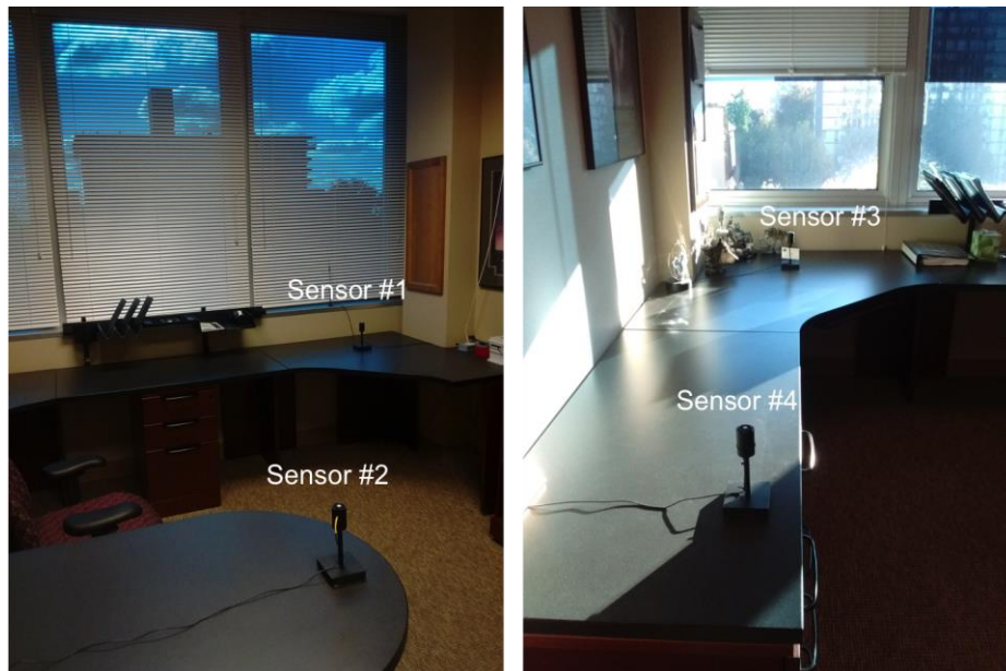
Figure IV-17. Space Type B instrumentation. The image on the left shows an unoccupied office where the blinds were kept fully lowered with the slats open. The image on the right shows an occupied office where the occupant lowered the blinds to over approximately 50% of the surface of the windows, with slats closed.
