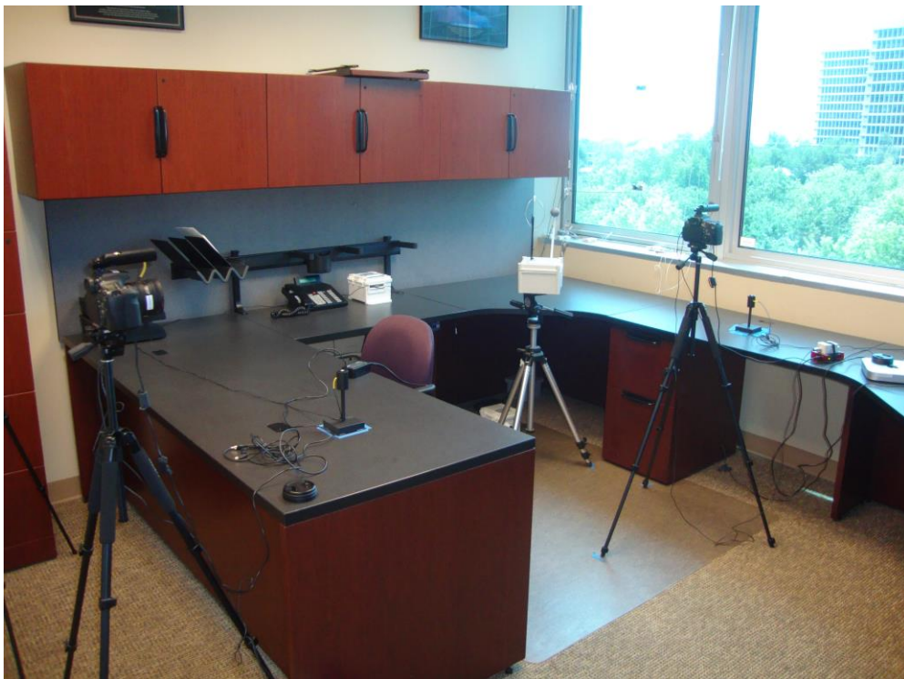
Figure IV-10. High-dynamic-range luminance mapping apparatus in operation at the study site (zone 18).
