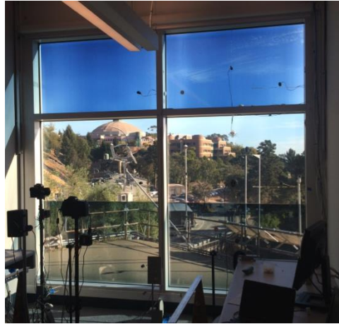
Figure IV-27. EC window in Room B when it was tinted, upper window transmittance = 1%, middle window transmittance = 60% and lower window transmittance = 18%.
