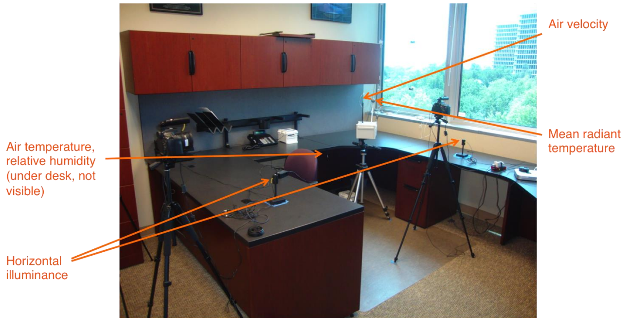
Figure IV-16. Instrumentation in Space Type A. Also shown are cameras in position for HDR imaging.
