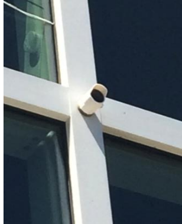
Figure IV-28. Exterior illuminance sensor was attached on the window frame of south façade.
