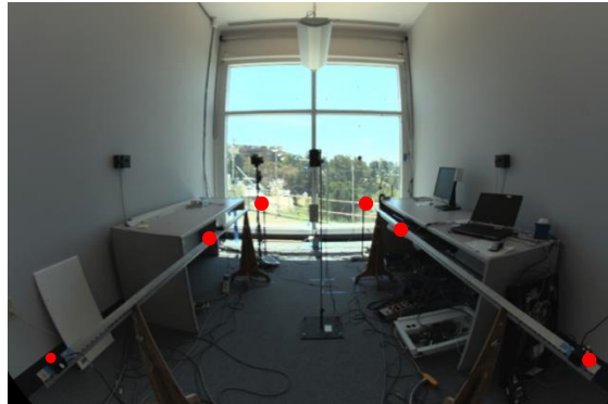
Figure IV-21. Illuminance sensor positions in a test room (red dots).
