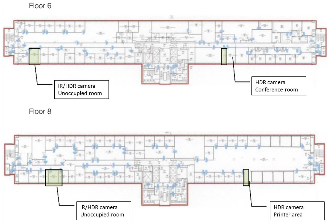
Figure IV.E.2. Locations of sensors on Floors 6 and 8 for the periodic site visits during the summer and winter solstices and the equinox.
