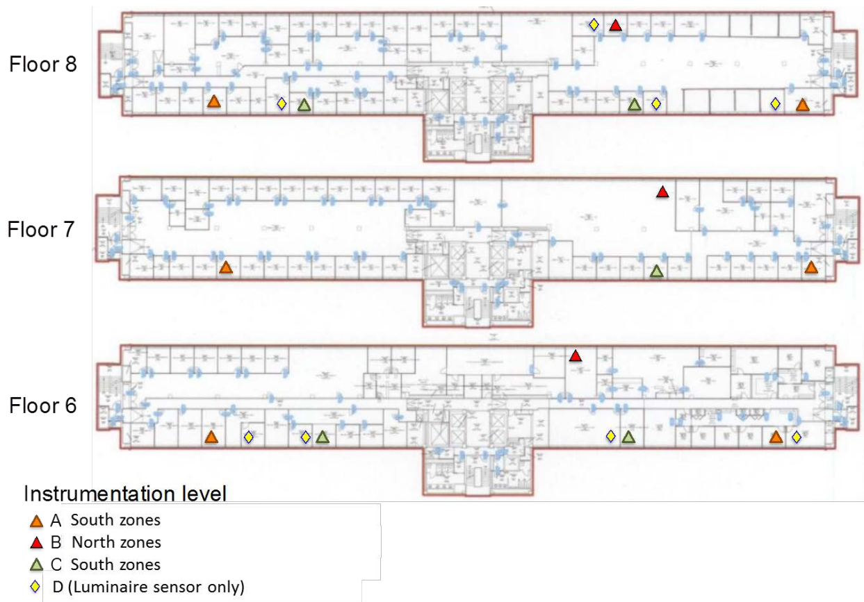
Figure IV.E.1. Locations of continuously monitored sensors on Floors 6–8.
