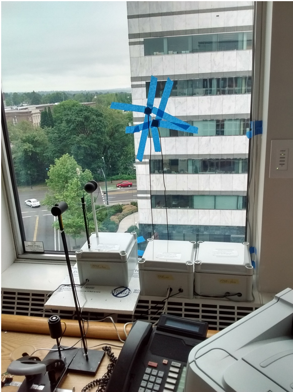
Figure C.1. Room with instrumentation level A. Image taken prior to completion of installation. In particular, blue masking tape was removed after silicon sealant was set.
