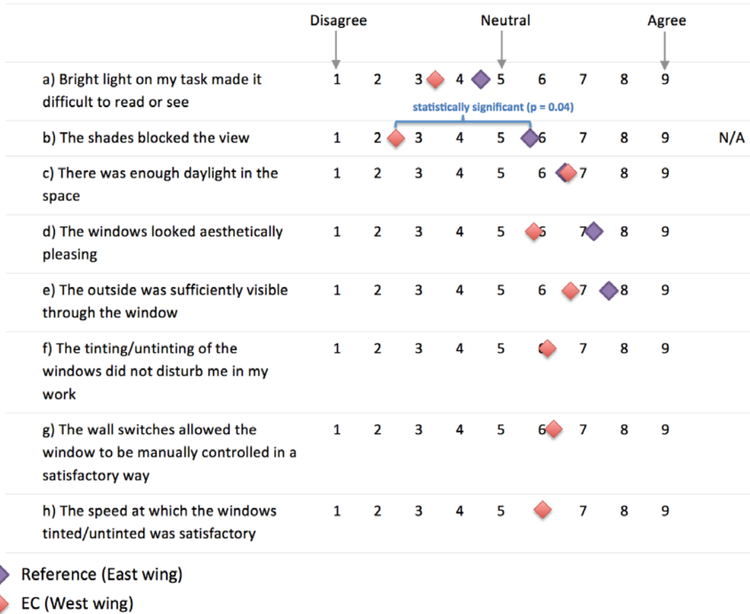
Figure V.G.7. Average occupant response regarding indoor environment on electrochromic (west) and reference (east) wings.
