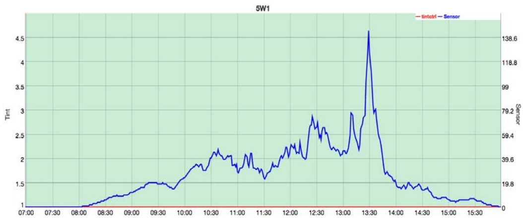
Figure V.C.9. Glare submode, Tint 3 max. Above: Daylight glare probability (DGP) for a view facing the window at seated height, 4 ft. from the south-facing EC or reference window. Below: EC tint level (red line, left y-axis) and outdoor vertical illuminance sensor (blue line, right y-axis) versus time of day. Data are given for December 22, 2015. Note: glare mode was not triggered for this day.
