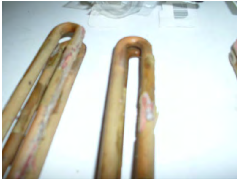
Figure 4. Heating Element Removed from the Electric Water Heater.
