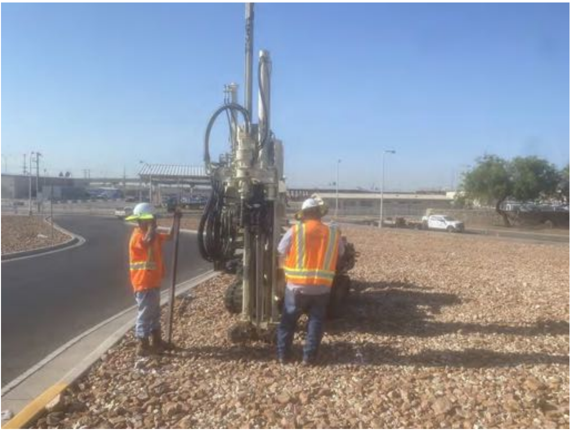
Photograph 1: View looking south of the drilling of soil boring SB-1 near the POE access road.
