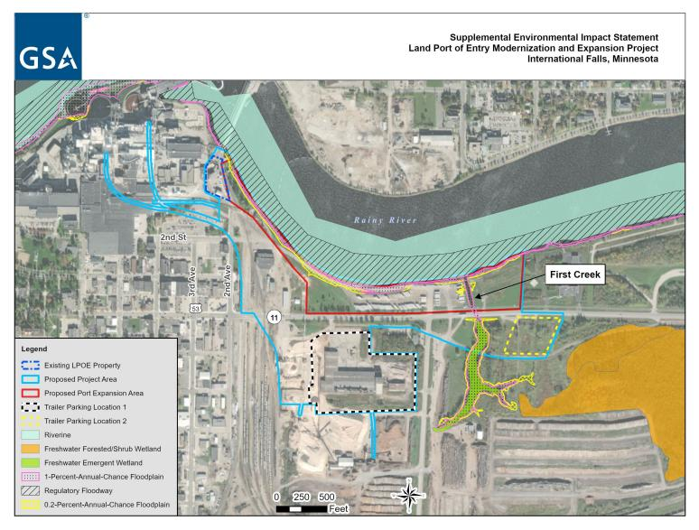
Note: The former culvert within the proposed expansion area that drains First Creek into the Rainy River currently is not classified as a wetland in the NWI; this segment was formerly covered, but then daylighted around 2013 because of the collapsed culvert.
