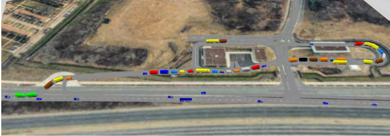
Figure 10. Simulated Queue on the Access Road at Gate 6 during 2018 AM Peak Hour with Alternative 3
