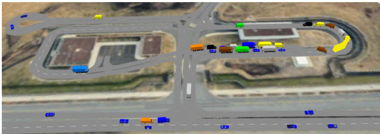
Figure 9. Simulated Queue on the Access Road at Gate 6 during 2018 AM Peak Hour with Alternative 2
