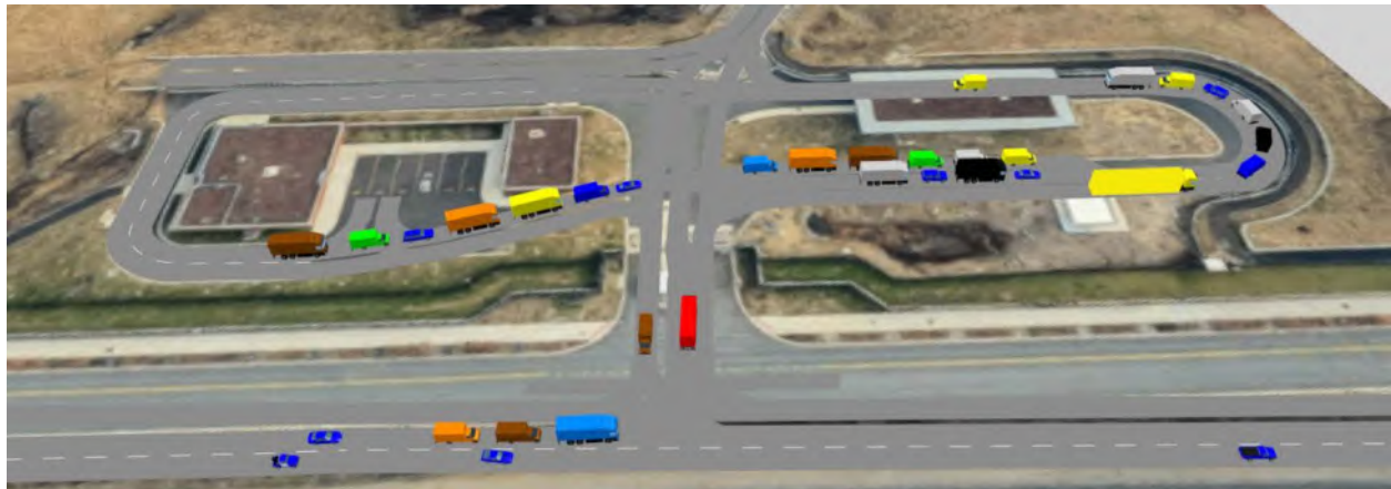
Figure 8. Simulated Queue on the Access Road at Gate 6 during 2018 AM Peak Hour with Alternative 1
