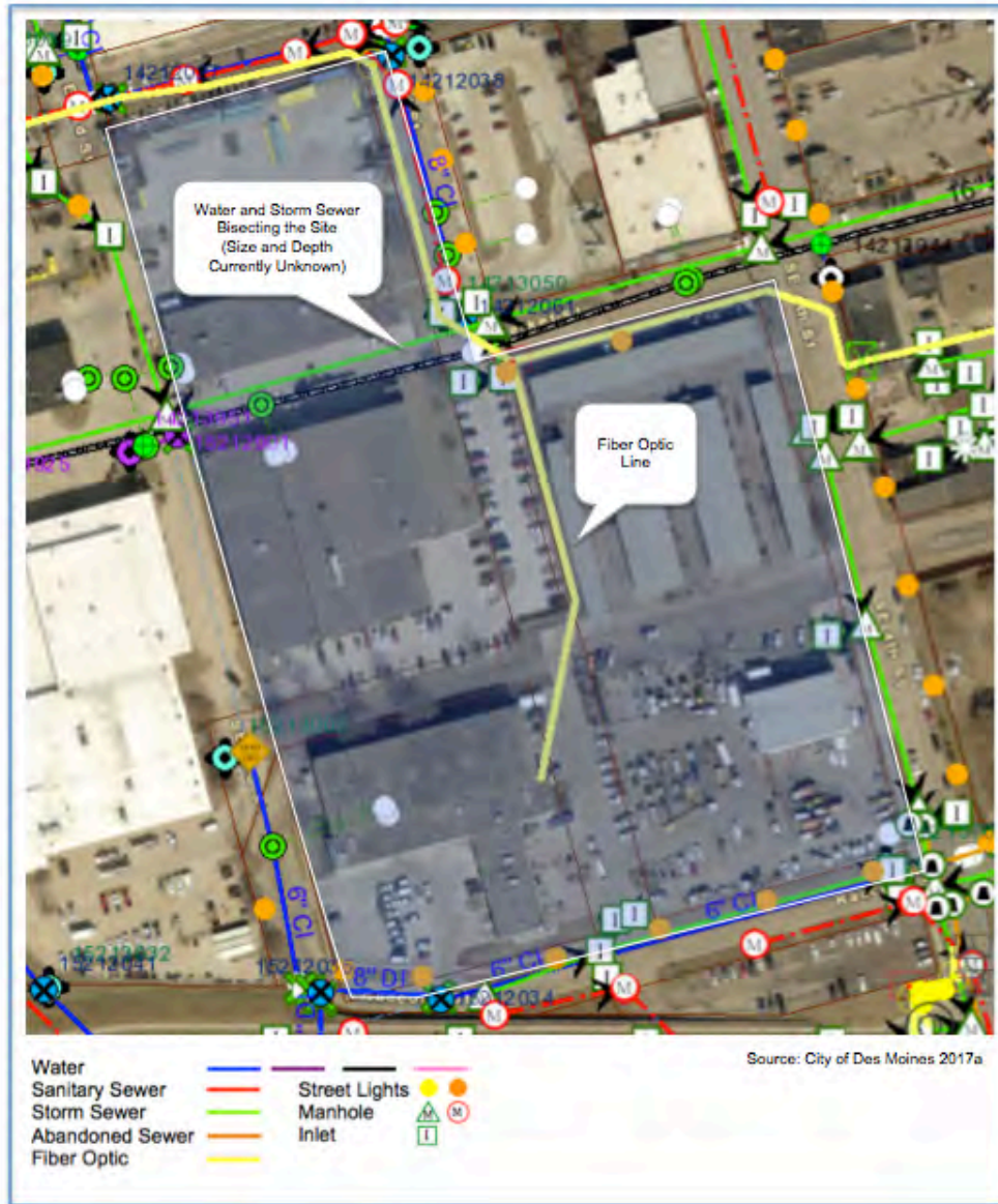
Figure 3-13. Water, Sanitary Sewer, and Storm Sewer Lines near the North MLK Site.
