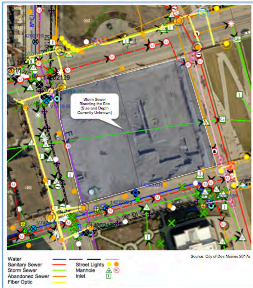
Figure 3-12. Water, Sanitary Sewer, and Storm Sewer Lines near the Former YMCA Site.
