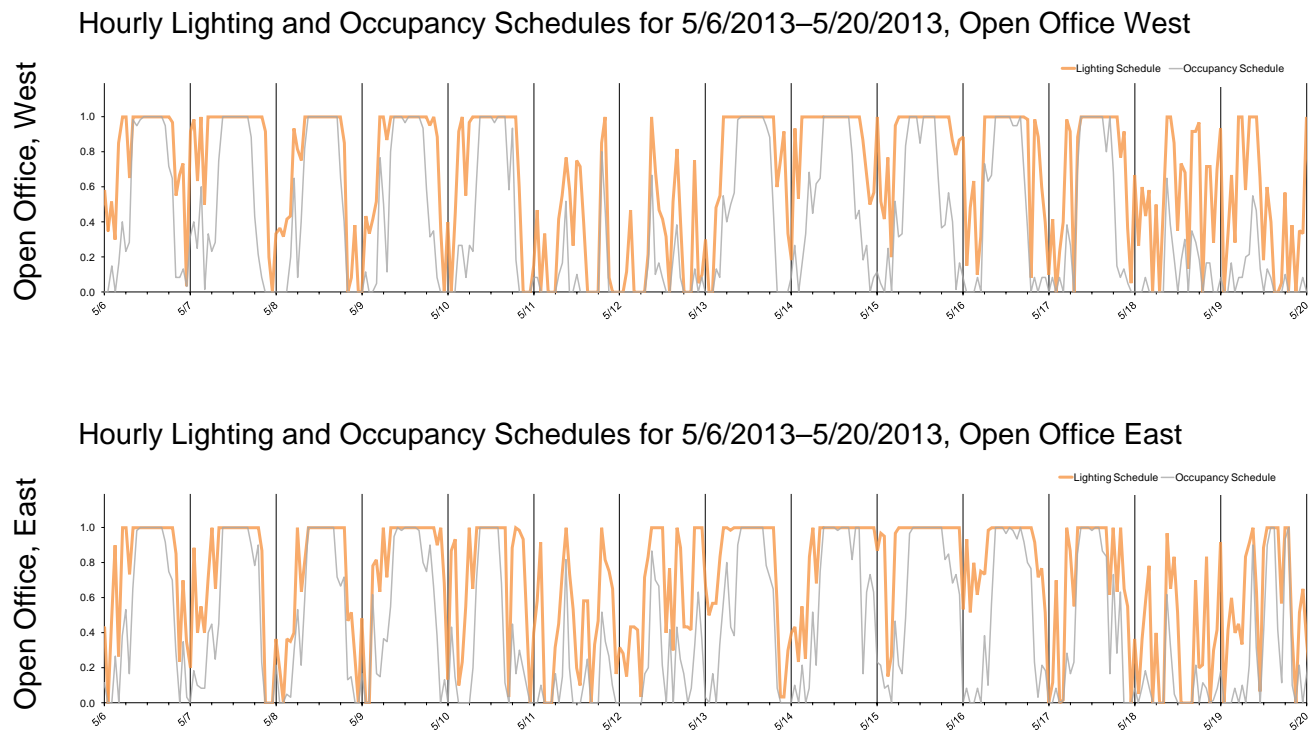
Figure 35 Measured Hourly Ambient Lighting and Occupancy Schedules for a Building 9447 High-Bay Module
