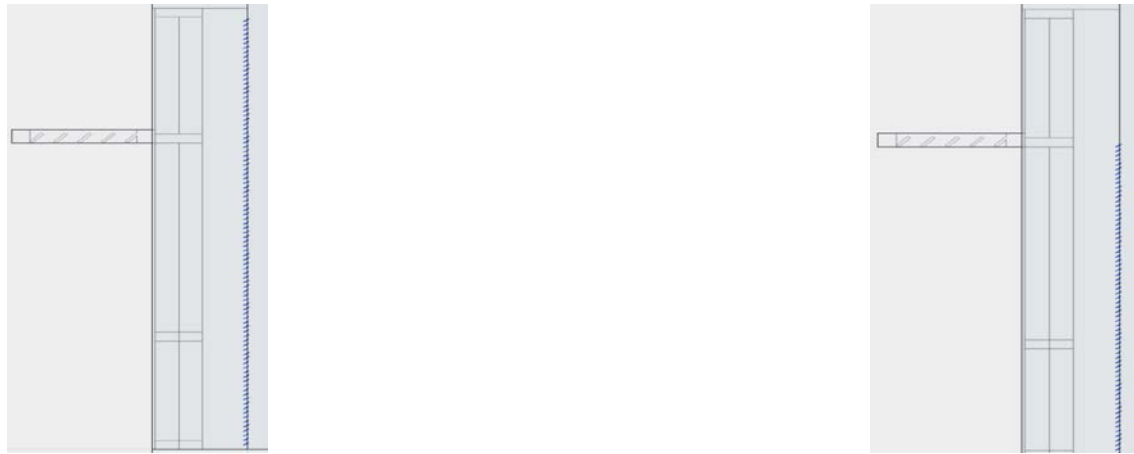
Figure 40 Building 9420 open office section (left) with the blind head height at the top of the vision glazing (right)
