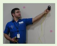
To compare the new LED lamp with the incumbent CFL, horizontal and vertical light levels were measured. A difference of less than 100 Lux is typically not noticeable by the human eye.
