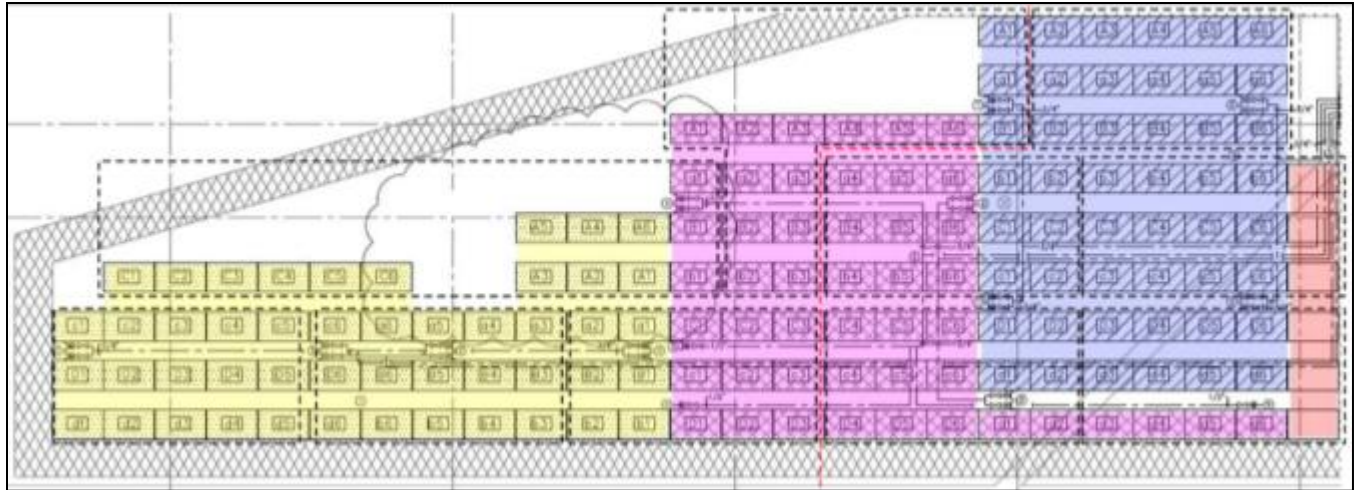
Figure 14. PV-T System solar thermal loops and 6 PV panels without solar thermal
