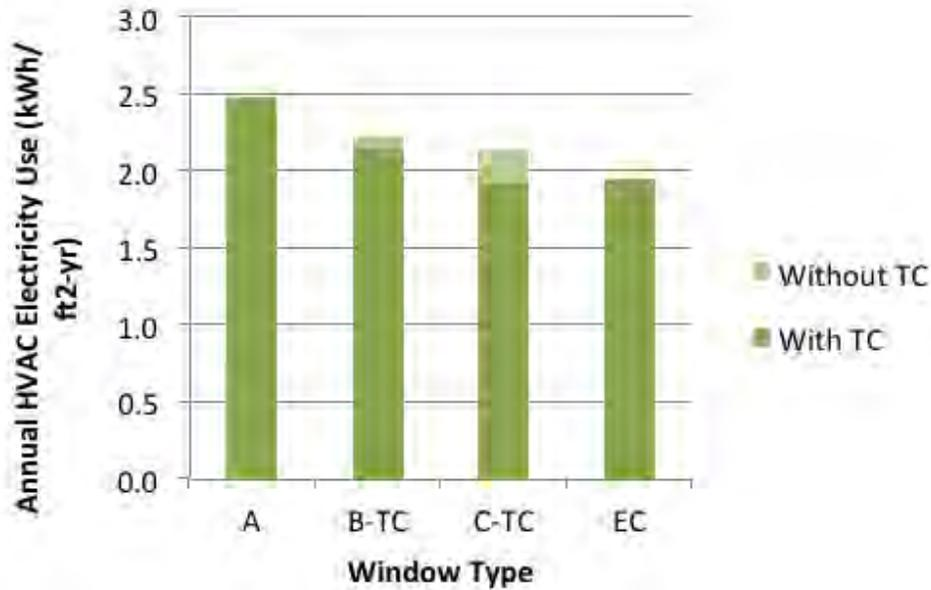
Figure 20: Annual HVAC electricity use for single-pane clear (A), window with and without TC film (B-TC), low-e with and without TC film (C-TC), and electrochromic window. Results given for the 48-ft deep west-facing perimeter zone in the Denver Federal Center, Denver, CO.
