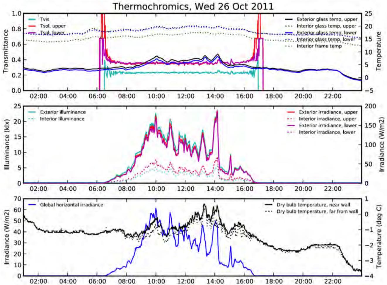
**Figure 9: Thermochromic window switching pattern on a cold overcast day (October 26, 2011). In this case, the thermochromic window stays unswitched throughout the day as indicated by the light blue line ( $T_{vis}$ ) in the top graph.**
