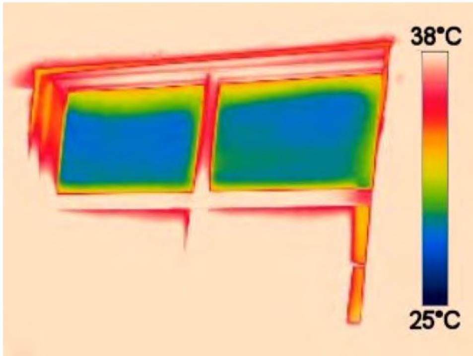
Figure 16: Infrared surface temperatures, no direct sun on the upper panes. Image taken September 22, 2011, 12:20 PM ST when the outdoor air temperature was 26°C.
