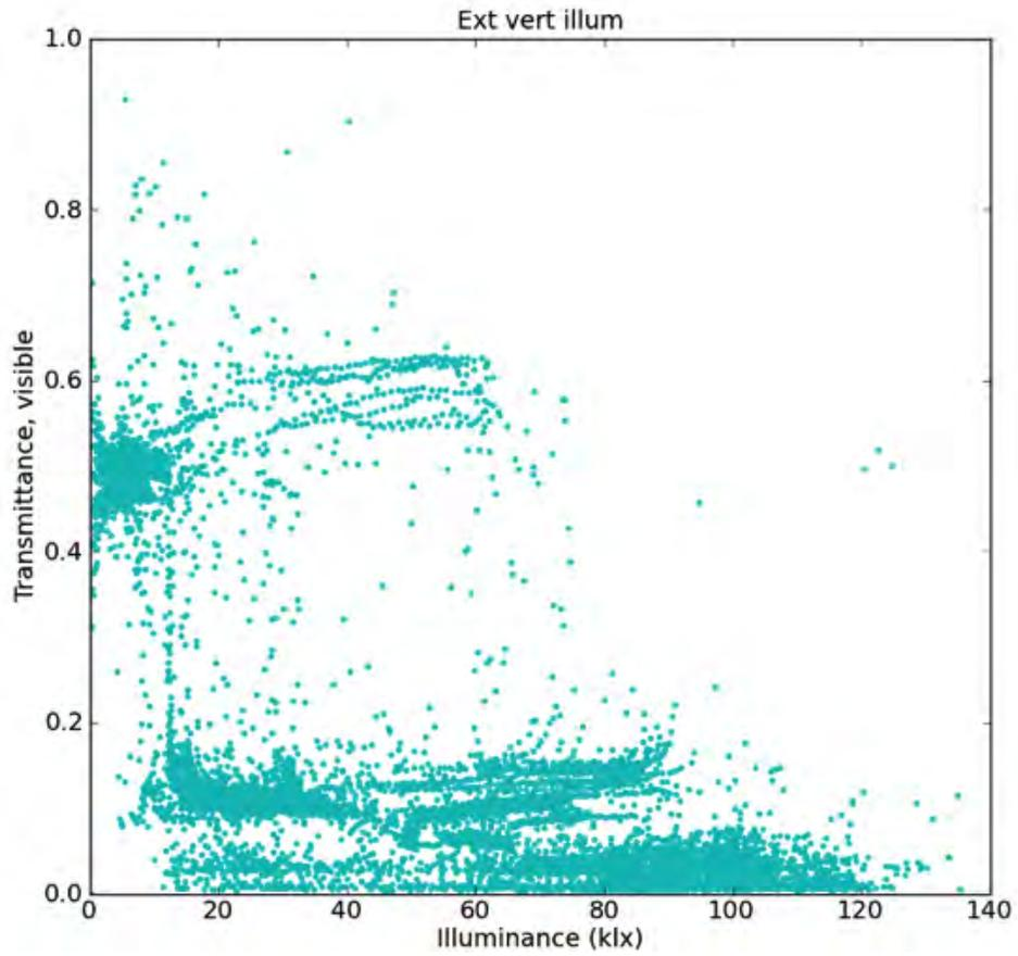
**Figure 26: Phase I nominal visible transmittance of the electrochromic window (y-axis) versus the exterior vertical illuminance (klux). As the outdoor illuminance increased, the daylight mode of the automatic controls decreased the tint level of the electrochromic window.**
