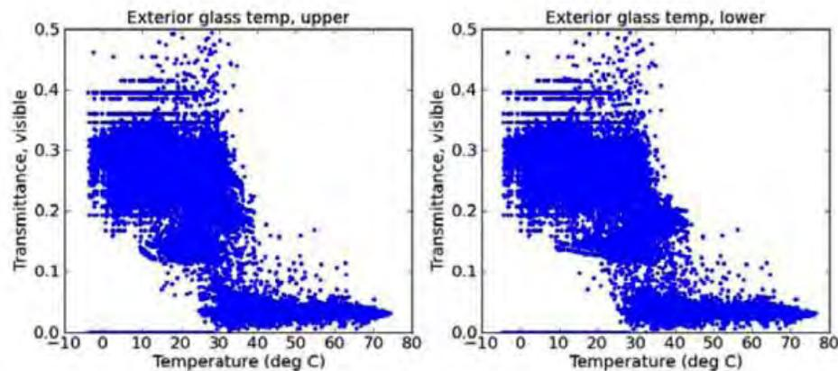
Figure 11: Nominal visible transmittance ( $T_{vis}$ ) of the thermochromic window as a function of exterior glass surface temperature, measured on the upper (left graph) and lower (right graph) lites.
