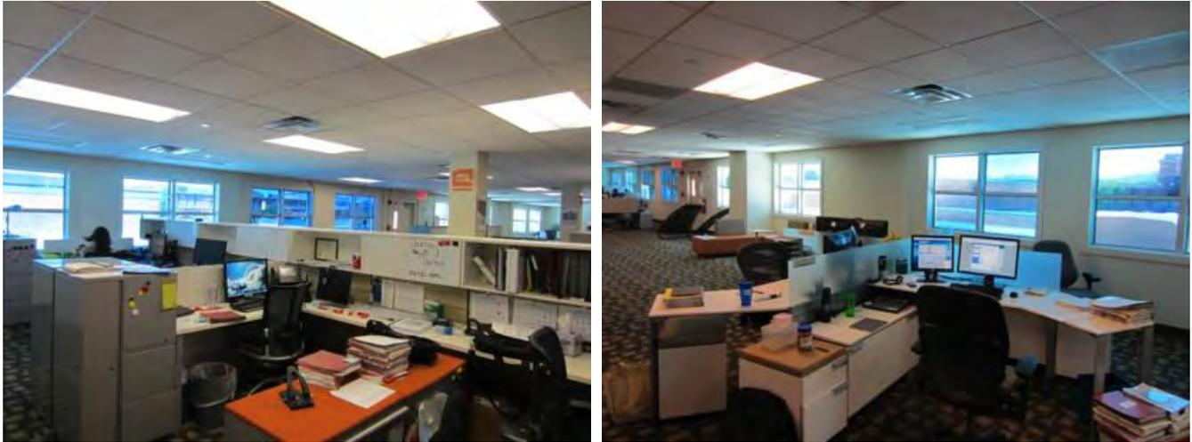
**Figure 4: Photograph of the perimeter zone during Phase II, where the existing furniture near the windows was replaced in January 2012 with low-height workstation furniture in the electrochromic area and part of the thermochromic area. Left: View of the south end of the electrochromic window area showing the linear high-efficiency workstation layout. Right: View from the north end of the electrochromic window area showing the high efficiency workstations serving four occupants.**
