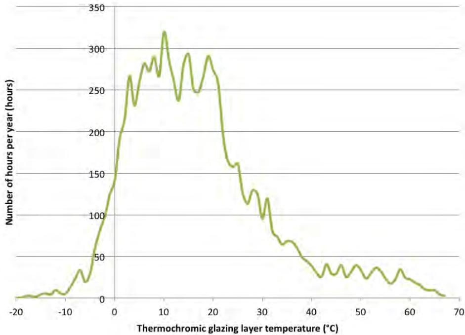
**Figure 22: Number of hours per year that the surface temperature of the thermochromic window was at a given temperature. For example, the thermochromic window was at a temperature of 32°F (0°C) for 150 hours in the year. Data were generated using EnergyPlus simulations.**
