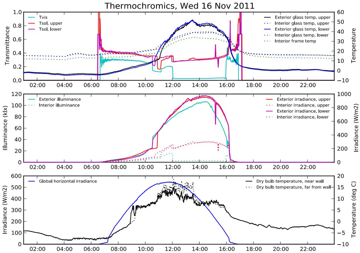
**Figure 8: Thermochromic window switching pattern on a cold, sunny day (November 16, 2011). Thermochromic in this case switches to tinted from noon until 16:00 ST as indicated by the light blue line (*T<sub>vis</sub>*) in the top graph.**
