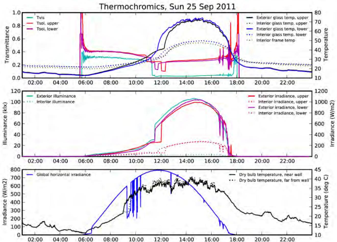
**Figure 7: Thermochromic window switching pattern on a warm, sunny day around the autumnal equinox (September 25, 2011). Notice how in the upper graph (light blue line), the visible transmittance ( $T_{vis}$ ) drops abruptly from a value of about 0.30 to 0.03 after around 11:00 in the morning. Time of day is shown on the x-axis (Mountain Standard Time). Nominal visible and solar transmittance data ( $T_{vis}$ ' ,  $T_{sol}$ ' ) are given on the**
