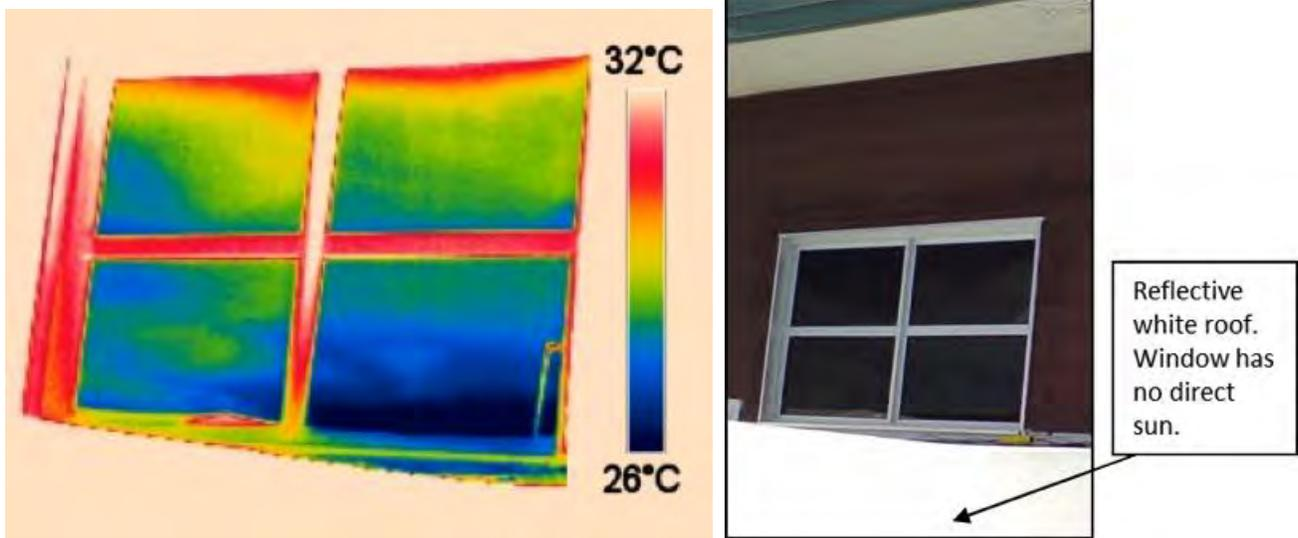
Figure 19: Infrared image (left) and photographic image (right) showing the thermal surface temperature patterns matching the switching pattern of thermochromic glazing when direct sun has not yet covered the upper panes. Images given for September 23, 2011, 11:03 AM ST.
