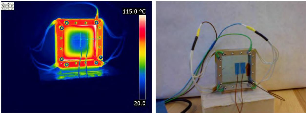
Figure B-1: Thermochromic sample heated at edges.
