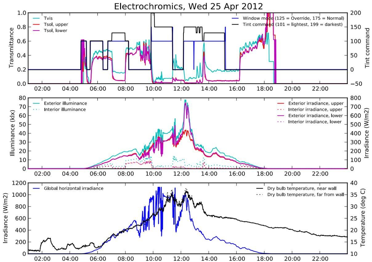
**Figure 30: Phase II electrochromic switching pattern on a cool then hot spring day (April 25, 2012). The HVAC control mode, indicated by the dark blue line in the top graph, is in effect when the tint command value is 125.**
