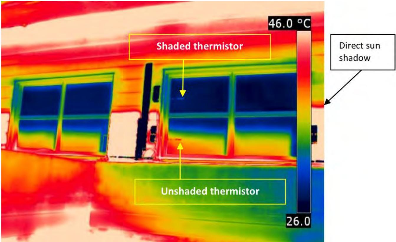
Figure 12: An infrared image of the dark tinted regions in the lower panes as the thermochromic transitions from clear to tinted with direct sun patches on the window. Image taken September 22, 2011, 11:57 AM ST.
