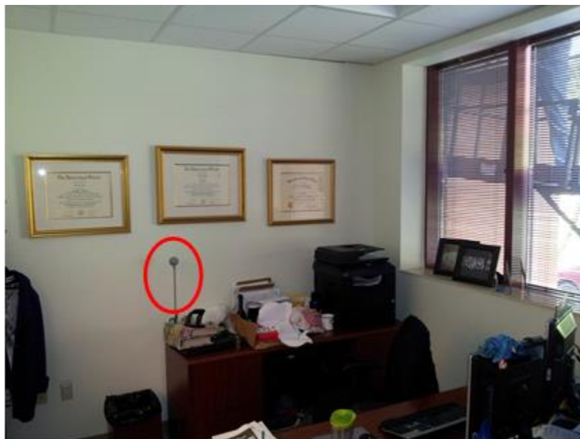
Figure 6. Globe temperature sensor on cabinet near occupant to measure effective radiant temperature, important to thermal comfort
