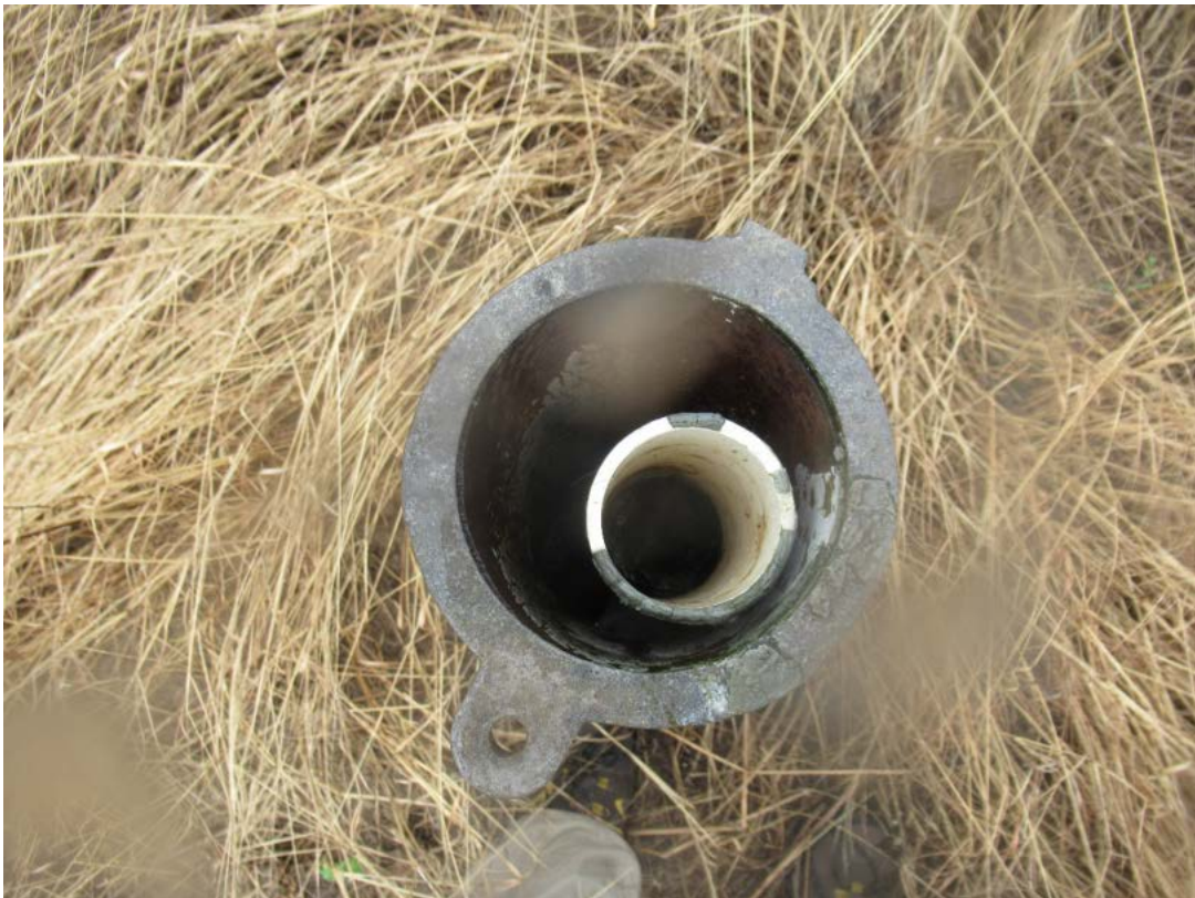
Photo 8: Open monitoring well at northeastern corner of the site.
