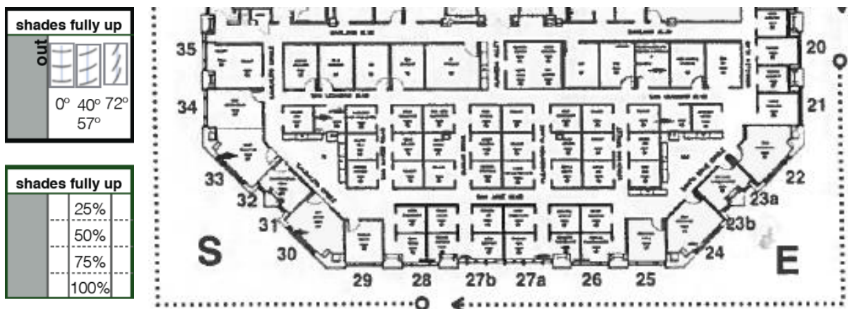
Figure 30. Left: Slat angle convention for upper shade (upper) and lower shade (lower). Right: Floor plan showing numbered GZSC shade locations at the OFB site. Windows 22, 25, and 29 were installed with the GG shade. The remaining windows were installed with the GS shade. Windows 25, 30 and 33 had the opaque backing on the vertical blinds prior to replacement with DZSC shades.
