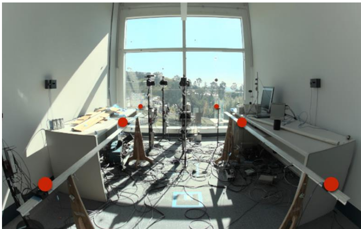
Figure 19. Photograph of B71T test chamber showing location of workplane illuminance sensors.
