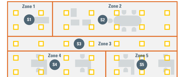
Figure 14 Sensors are Mounted External to Luminaires in Zone-Based Control
