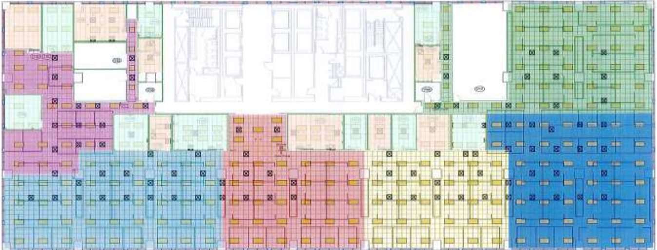
Figure 12: Metcalfe LED fixture control groups programmed during system commissioning
