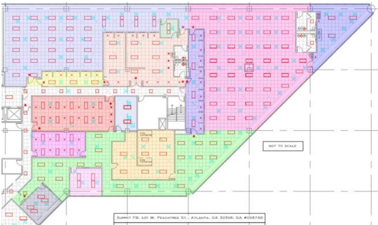
Figure 13: Summit LED fixture control groups programmed during system commissioning
