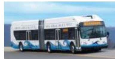
Name: New Flyer XFC60 (FCEV) SIN: 377F Price: $1,742,200 Incremental Cost: $1,227,858 Range: 240 miles
