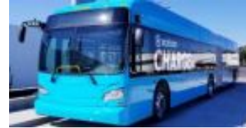
Name: New Flyer XBE60 SIN: 377E, 377I Price: $1,517,385 Incremental Cost: $1,005,247 Range: 153 miles
