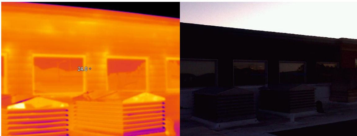
Figure 18: IR image (left) of the two quad-pane windows outside and the visual photo (right) of the same location (Credit: Ed Hancock)
