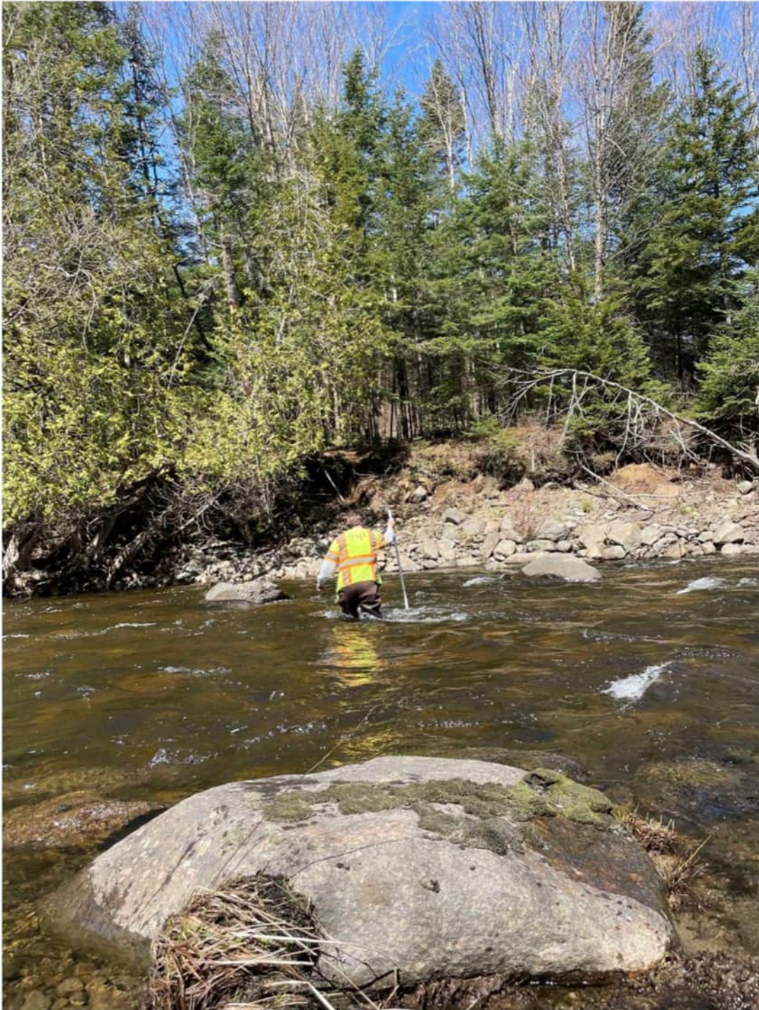
5. Field staff collecting depth measurements at Transect T2.
