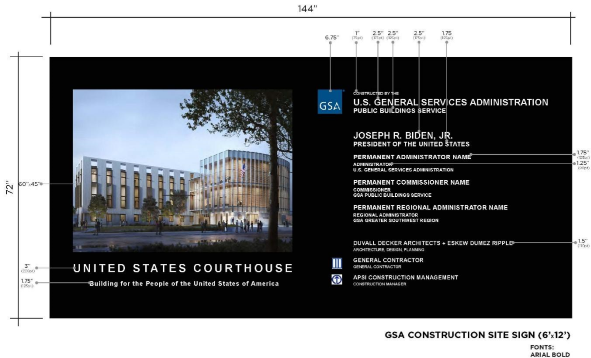
Figure 5: Construction Sign Example
