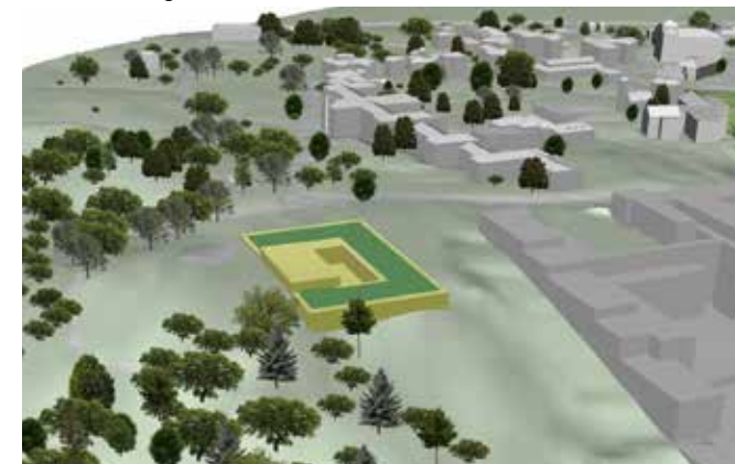
Study 3. Reduce Headhouse to 1 story and relocate to the north of the site, aligned with Munro. Below grade building may shift east or west. Rotate the below-grade structure to maximize solar access and to reduce the frontage facing the cemetery.
