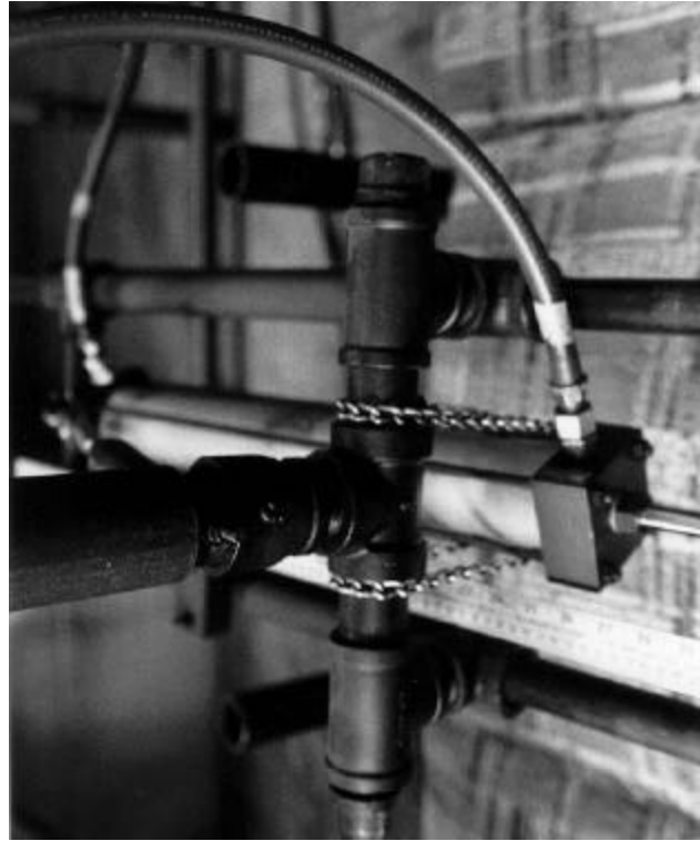
Figure 11. Crossed Tees attached to the free ends of the extension shaft sleeve bearings in the external load frame together with a Tee attached to the lower end of the vertical swivel support column and a one inch diameter cross shaft or hinge pin which passes through them to form a hinge which allows the backrest load frame to pivot up and down.
