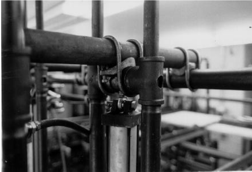
Figure 7b. The load frames are attached to the main testing machine frame as shown here.
