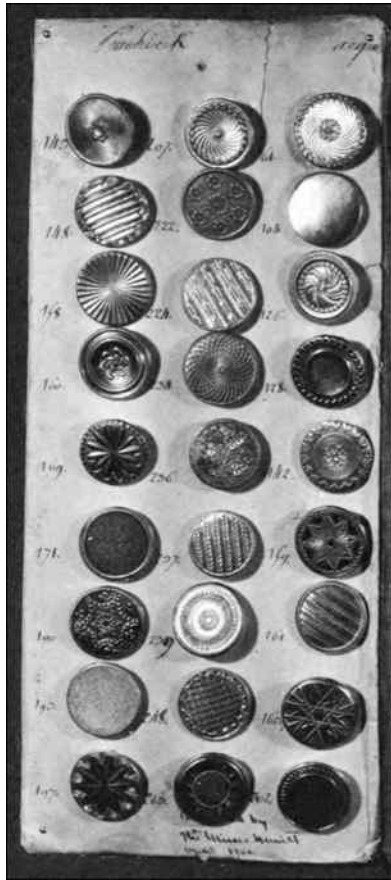
Figure 141. Example of a salesman's sample card, circa 1780, for buttons made from pinchbeck, a copper alloy that retains its polish (source: Albert and Kent 1949:392).
