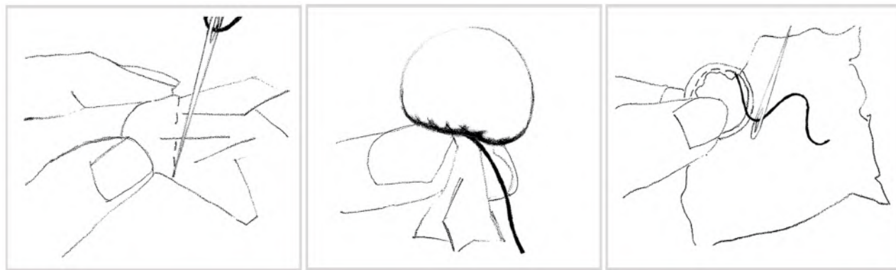
Figure 143. Diagram showing the process for covering a button blank or button ring with cloth (drawing by Alliah Humber).
